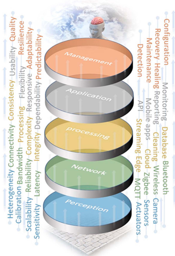
FIGURE 1. Various layers of the Internet of Things (IoT) architecture, starting from the perception layer where the data are generated, advancing through the communication and computing stages as well as storing data, and culminating in a decision. API: application programming interface.
