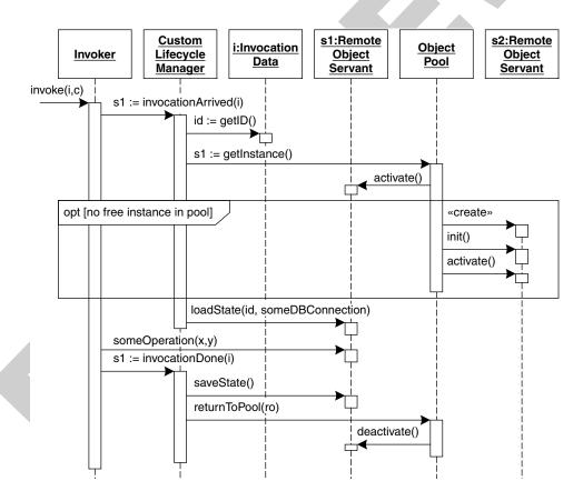
In the figure above the LIFECYCLE MANAGER obtains a servant from a pool of servants. After the servant is activated (or optionally created lazily), the state associated with the given OBJECT ID is loaded from persistent storage. The operation is executed, and finally the state of the remote object is passivated and the servant is put back into the pool.
