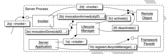
A LIFECYCLE MANAGER is typically created by the server application during start-up, and is registered with the distributed object middleware's INVOKER. Before an invocation is dispatched, the INVOKER informs the lifecycle manager. If the servant is not active, the LIFECYCLE MANAGER activates it. The INVOKER dispatches the invocation. After the invocation returns, the LIFECYCLE MANAGER is informed again and can deactivate the servant if required.
