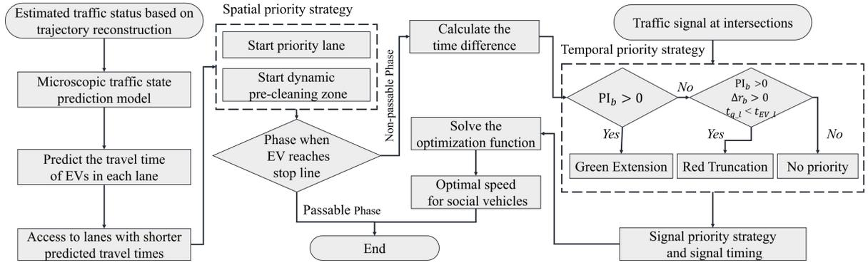
Fig. 6. The process of EVP based on the MPC controller
