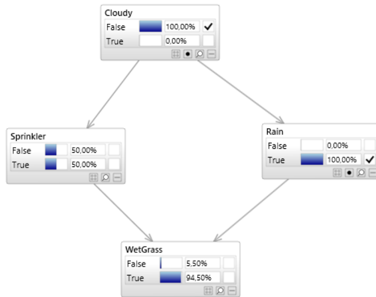
Figure 2.2: A structure of a simple Bayesian Network designed using Bayes Server, version 5 [83]
