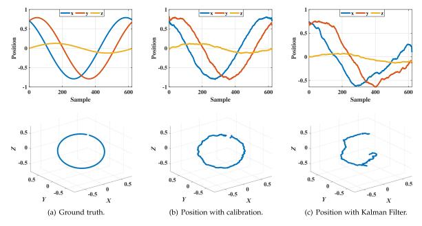
Fig. 8. Three-axis position (first row) and trace (second row) of our opportunistic calibration and Kalman filter.
