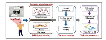
Fig. 5. System architecture of IA-Track.
