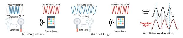
Fig. 7. IA-Track uses signal compression or stretching phenomenon for distance calculation.
