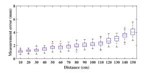
Fig. 11. Ranging accuracy interconnected with smartphone.
