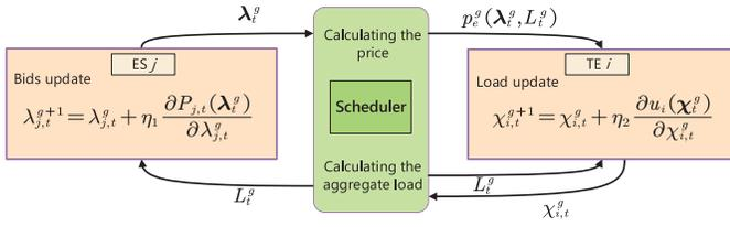
Fig. 4. Interactions between the ESs, TEs and scheduler.
