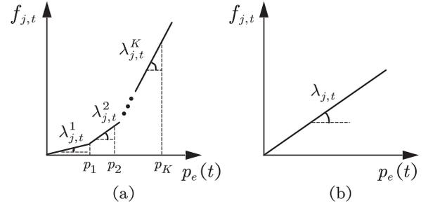
Fig. 3. (a) Piece-wise linear. (b) Affine supply functions.
