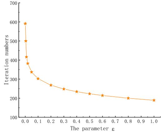
Fig. 14. The influence of the parameter  $\epsilon$  on iteration numbers.
