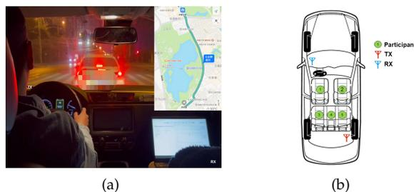
Fig. 14: Car experiment scene: (a) Passenger counting test in a 5-seat SUV. The total length of the test section is 1.7 kilometers, and the average test speed is 35km/h. (b) Seating configuration: The five positions in the car (including the driver's seat) are numbered 1-5 in sequence, and are divided into 8 seat configurations according to the number of people and usage habits.
