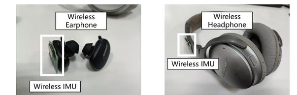
(a) Wireless earphone taped with a wireless IMU. (b) Wireless headphone taped with a wireless IMU.
