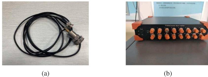
Fig. 10. Schematic diagram of acceleration sensor and signal acquisition card: (a) acceleration sensor; (b) signal acquisition card.
