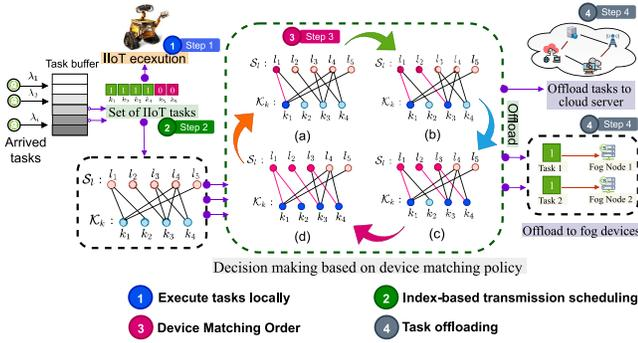
Fig. 4. Illustration of the proposed computation offloading strategy.
