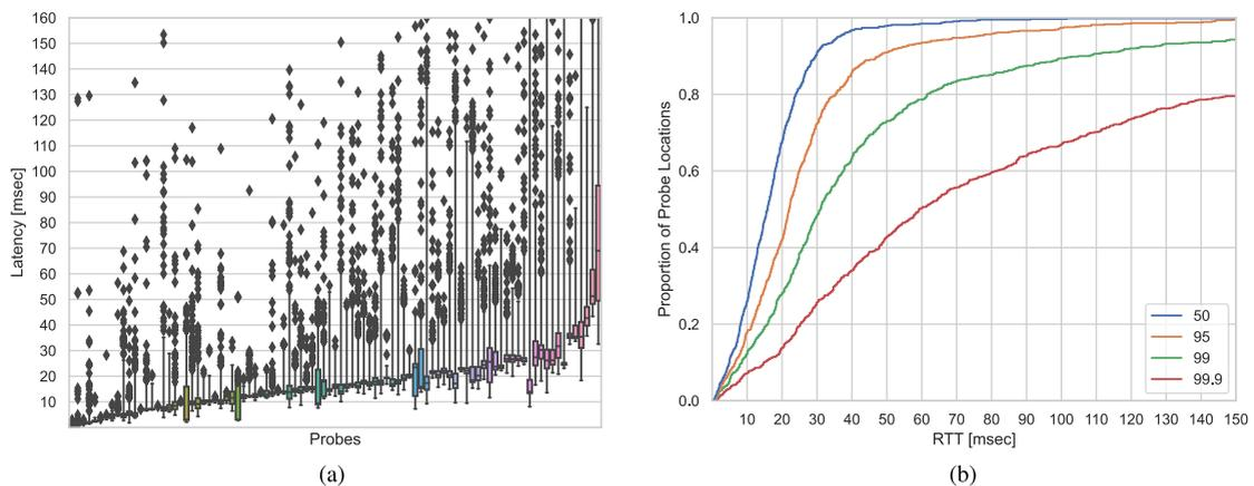
**FIGURE 1.** Latency to closest cloud data center for probe locations in the USA with at least 100 measurements. (a) Boxplot of probe location latencies shorter in order of increasing average latency. Whiskers show minimum and 99% latency. (b) CDF of latencies for probe locations.
