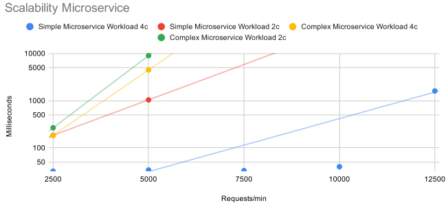
Figure 9 Changes in the response time per number of requests for the microservice system in the experiment 1.
