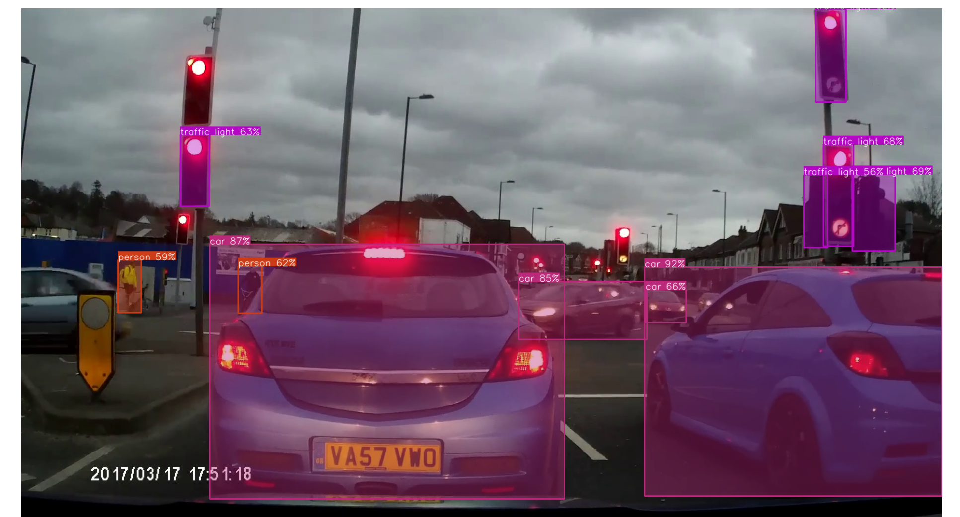
Fig. 1: Processing video frames with YOLOv8 to analyze traffic; computation occurs at nearby edge devices with low latency
