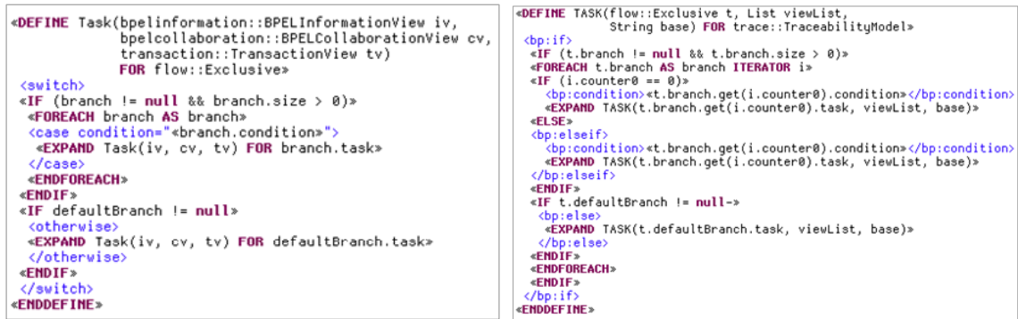
Figure 6.12: Adjusting transformation templates for generating process code in new technology
