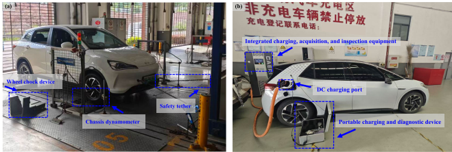
Fig. 4. Experimental setup for capacity ground-truth calibration. (a) Discharge test environment chamber and (b) charge test environment chamber.
