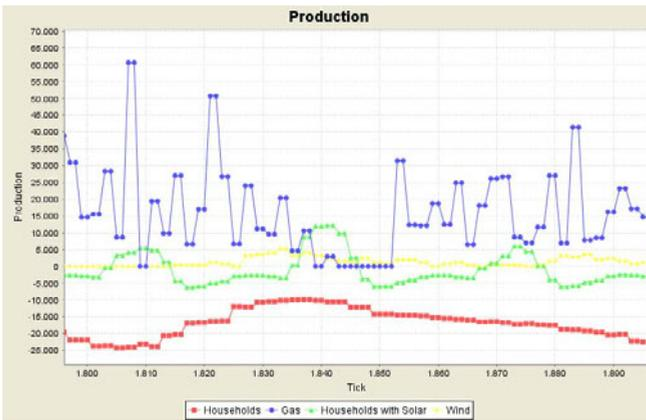
Fig. 3. Response in the curves for increased solar energy production
