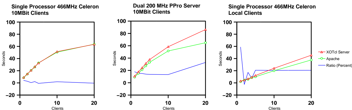
Figure 14: Comparison of the xOComm-HTTP Server vs. Apache 1.3.6
