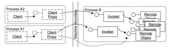
The CLIENT PROXY sends a request to the INVOKER with invocation information for a REMOTE OBJECT. The INVOKER dispatches the local object address and operation implementation. Then it invokes the correct operation implementation for this object.
