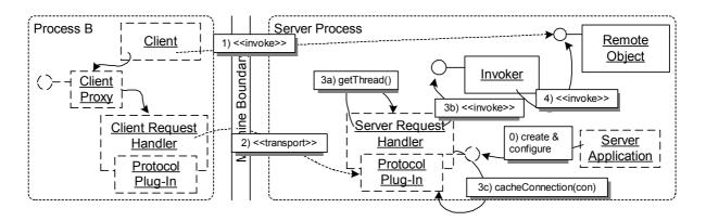
The SERVER APPLICATION creates and configures the PROTOCOL PLUG-IN for the RE-QUEST HANDLER. For an invocation, the CLIENT PROXY transports the message to this PROTOCOL PLUG-IN. The REQUEST HANDLER then forwards the invocation to the IN-VOKER. It may cache the connection in the PROTOCOL PLUG-IN.
