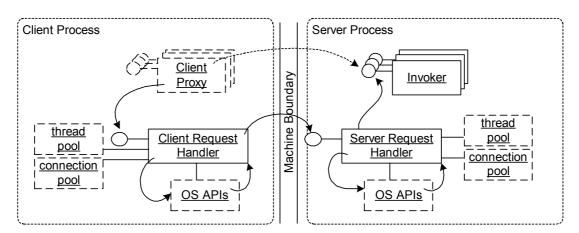
Connections are handled by the REQUEST HANDLER on client and server side. These are used by CLIENT PROXIES and INVOKERS. The REQUEST HANDLER makes effective use of the communication resources and the operating system APIs, and it pools connections handles and threads.
