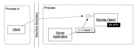
The SERVER APPLICATION instantiates a REMOTE OBJECT. Then clients can access the RE-MOTE OBJECT using the functionality provided by the distributed object framework.
