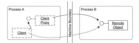
To invoke an operation of a REMOTE OBJECT, the client invokes a operation of the CLI-ENT PROXY that supports the REMOTE OBJECT'S interface. The CLIENT PROXY forwards this invocation to the REMOTE OBJECT. It handles the details of crossing the machine boundary and process boundary.
