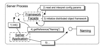
A FRAMEWORK FACADE is initialized by a SERVER APPLICATION. It reads and interprets the configuration parameters. Then it initializes the distributed object framework. It also serves as the central place to obtain references to central services, such as *naming*.
