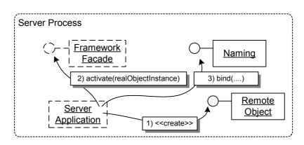
For each REMOTE OBJECT to be instantiated, the SERVER APPLICATION creates the object according to the activation strategy, activates it in the distributed object framework, and optionally binds it with *naming*.
