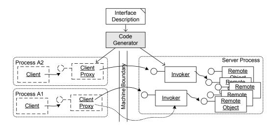
Using an INTERFACE DESCRIPTION in a separate file a code generator generates code for CLIENT PROXY and INVOKER. The CLIENT PROXY is then used by the client. It contacts the INVOKER that dispatches the invocation to the REMOTE OBJECT. This way, details of the distributed object framework are hidden from client and REMOTE OBJECT developers, as they only see client code, INTERFACE DESCRIPTION and REMOTE OBJECT code.
