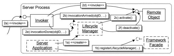
The responsible LIFECYCLE MANAGER is created by the SERVER APPLICATION during startup and it is registered with the distributed object framework using the FRAME-WORK FACADE'S API. Before an invocation the LIFECYCLE MANAGER is informed by the INVOKER. If the REMOTE OBJECT is not active, the LIFECYCLE MANAGER activates it. Then
