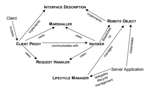
In most distributed object frameworks, these patterns are integrated with a few typical components. A SERVER APPLICATION instantiates and controls the REMOTE OBJECTS. The FRAMEWORK FACADE shields the distributed object framework and provides a simple API to developers using the distributed object framework.
