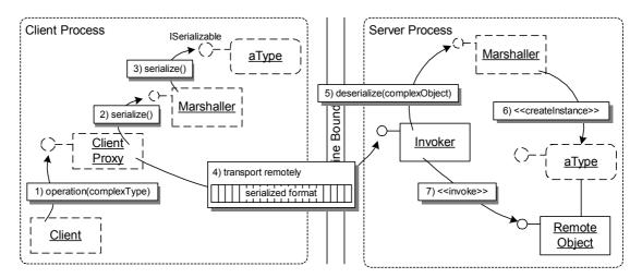
An operation with an object as argument is invoked. The CLIENT PROXY uses the responsible MARSHALLER to serialize this object. The serialized format is transported across the network. This format is de-serialized by the MARSHALLER on server side and the instance of the respective type is created. Finally, the REMOTE OBJECT is invoked and uses this object.
