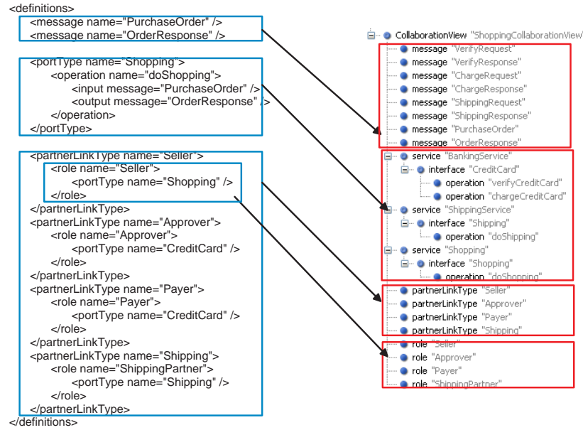
Fig. 6. The mapping of the Shopping process descriptions in WSDL to the collaboration view.
