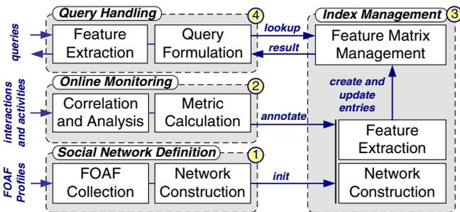
Fig. 4. Approach to feature-based discovery: (1) network definition, (2) network annotation, (3) feature index management, and (4) query handling.
