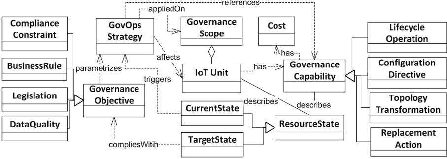
Fig. 2. Simplified UML diagram of GovOps model for IoT cloud governance.
