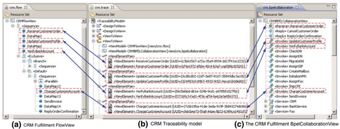
Fig. 15 Illustration of establishing trace dependencies ( middle ) of an integration of CRM FlowView ( left ) and BpelCollaborationView ( right )
