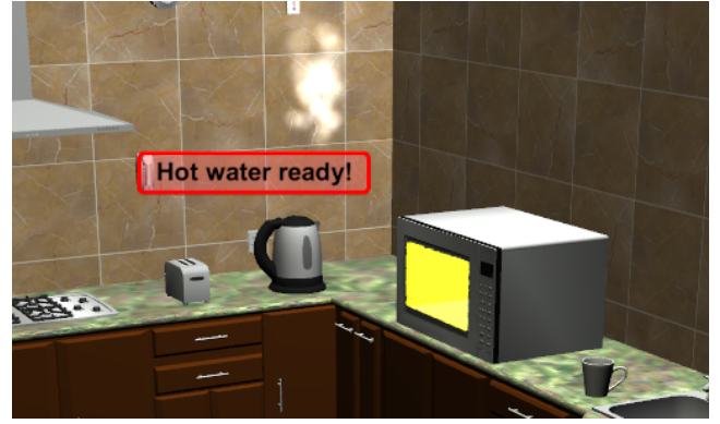
Figure 6: 3D scene of the real-world on the Web browser: the microwave oven will be in a highlighted status (yellow) while it is being used; a steam is shown on the kettle icon when the real kettle in the kitchen is boiling water.
