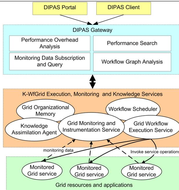
**Fig. 2.3** Overall architecture of the distributed performance analysis service (DIPAS). Arrowed black lines indicate the invocation of service operations (control and data flow). Arrowed dash lines indicate data flows.
