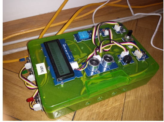
Fig. 7. An example of our gateways for Building Management Systems.
