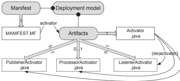
Fig. 10. DSL deployment model and artifacts
