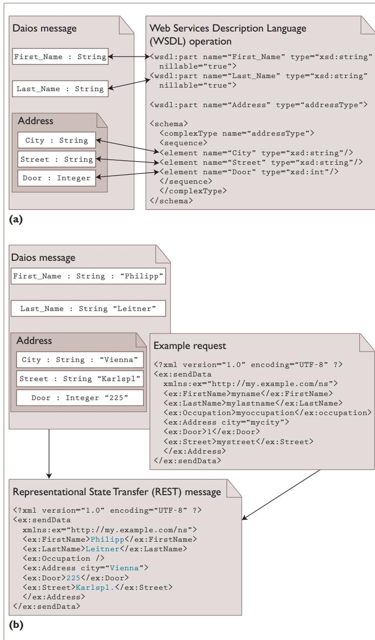
interface at all. If the user gives an example request, Daios uses the example as a template, which it fills with the user's actual input at invocation time, and issues an HTTP post request with the filled template as payload. If no information about the service interface is given (that is, neither WSDL description nor example request), Daios issues an HTTP get request with URL-encoded parameters.
